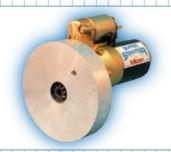
For use in custom applications. Mounting nose to be machined by customer. Includes 9-tooth, 12 pitch pinion gear.
