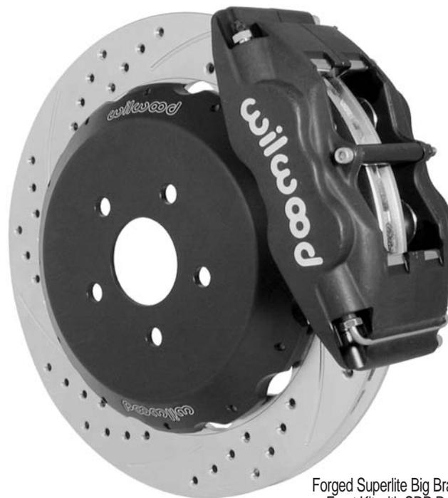
Forged Superlite Big Brake Front Kit with SRP Rotor
