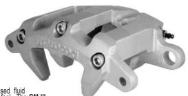
The **GM III** incorporates standard Wilwood features like stainless steel pistons for increased fluid protection and high temperature seals for controlled retraction which provides improved driver feel. The **GM III** for 1,00" width rotor is machined and fitted with OEM type slide pin vibration dampeners for a direct OEM caliper interchange.
