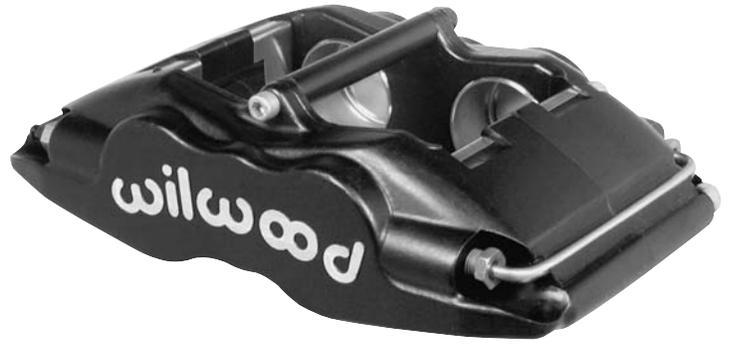
The most noteworthy feature of this new caliper design is the forging. Each body is stress-flow forged from premium grade aluminum alloy billets. Stress-flow forging re-aligns the metal's internal grain structure to flow within the contour of the caliper body. This process eliminates the stresses and interruptions to the internal grain structure that occur when machining a straight block billet. Simply stated, there is no better way to build a stronger aluminum caliper body.
