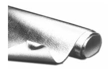
For conductive heat applications, the fabric side can handle temperatures in the range of 350-1200 degrees F. The highly reflective metallic surface is capable of withstanding radiant temperatures of up to 2000 degrees F. When used as a heat shield, the barrier should be installed so the bright metallic surface faces the heat source.
