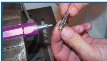
STEP THREE Insert olive on tube and under braid.
