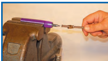
STEP ONE Insert hose on arbor.
