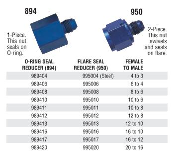
894 Series - Female side seals against o-ring and flange on mating male fitting. 950 Series - Female side seals internally on flare nose of mating male fitting. NO O-RING NECESSARY.
