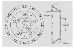
mount rotors provide the most durable and accurate method of isolating potential pad engagement harmonics and the in-service thermal variations that occur between the hat and the rotor.
