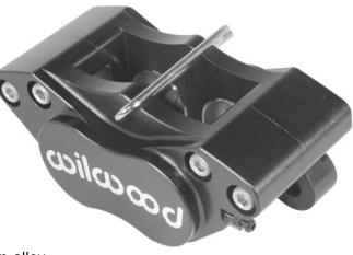
The **GP 320** is full CNC detail machined from premium alloy billet. FEA structural analysis technology was employed to develop a design that minimizes weight and maximizes rigidity against
