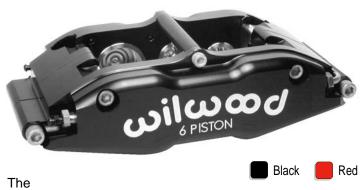
**SL6R** is well matched to the fluid output capabilities of many OE master cylinders and serves as the base caliper for Wilwood's 14.00" rotor front "Big Brake" conversion kits.
