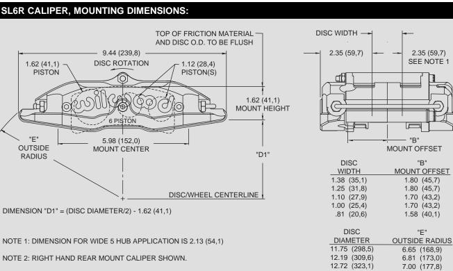
INLET FITTING: 1/8-27 NPT RADIAL MOUNT BRACKETS ARE AVAILABLE
