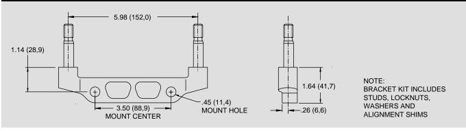
RADIAL CALIPER TO LUG MOUNT ADAPTER BRACKET, PART NUMBER 250-6308:
