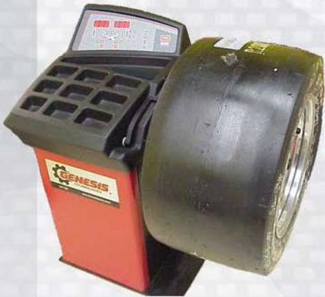
Balance all types of steel or light alloy wheels for cars, off-road vehicles and light commercial vehicles with high precision.
