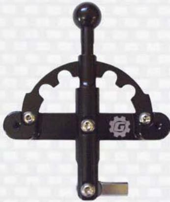
The 5 Way Sway Bar Controller is machined from 6061-T6 aluminum and features a female threaded rod end for the control cable connection. Deep machined grooves ensure a positive engagement and will not slip out of position due to vibration or accidental contact.
