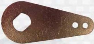
The Sway Bar Blade Crank Plates are laser cut from 1/8" mild steel and nickel plated for additional protection from the elements. Two location holes are provided for the control cable attachment.
