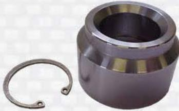
This mild steel Lower Ball Joint Housing is perfect for racers wanting to build replacement A-Arms. Simply weld your steel arms to the housing to complete the A-Arm structure. The housing is designed for a 0.75" mono ball bearing, and has a snap ring groove for bearing retention.
